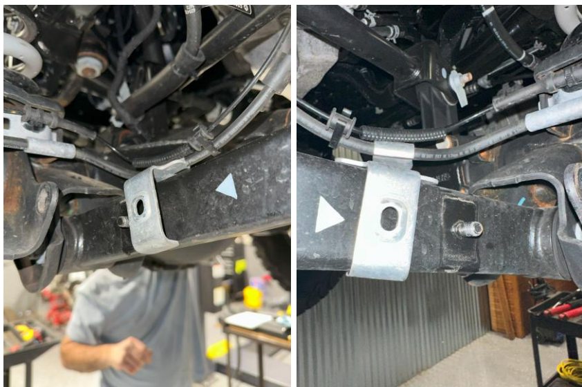
Figure 6: Front driver/passenger lower brake line mount removed
