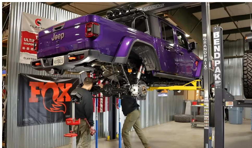
Figure 19: Rear tires removed, axle drooped
