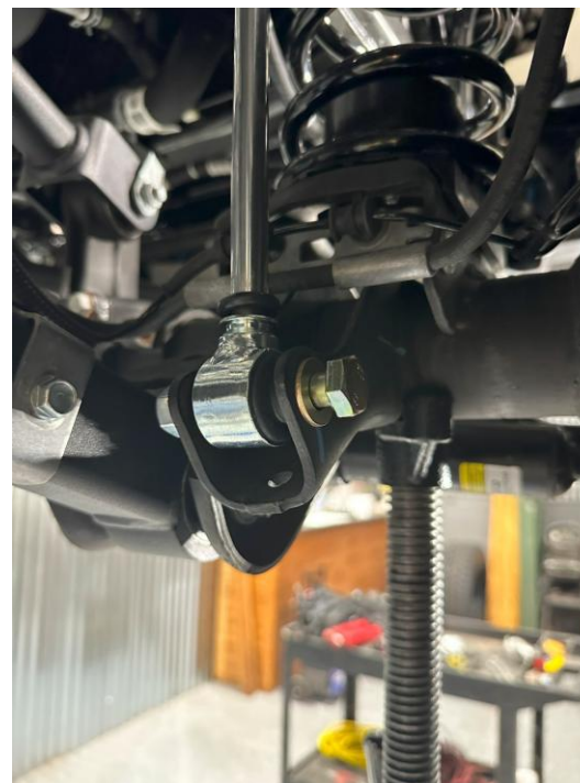
Figure 12: Front shock top and bottom bolt installed loosely
