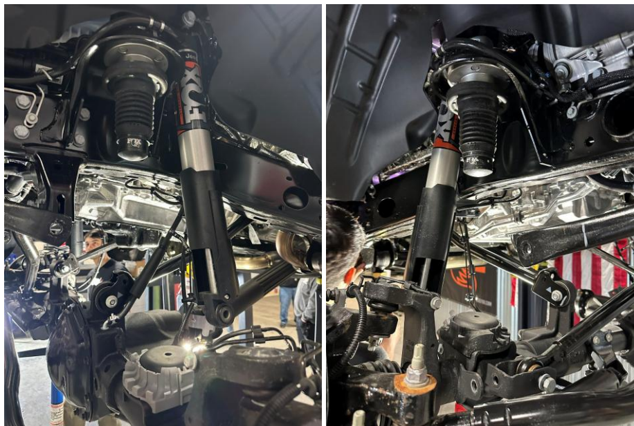
Figure 10: Axle drooped with old springs removed
