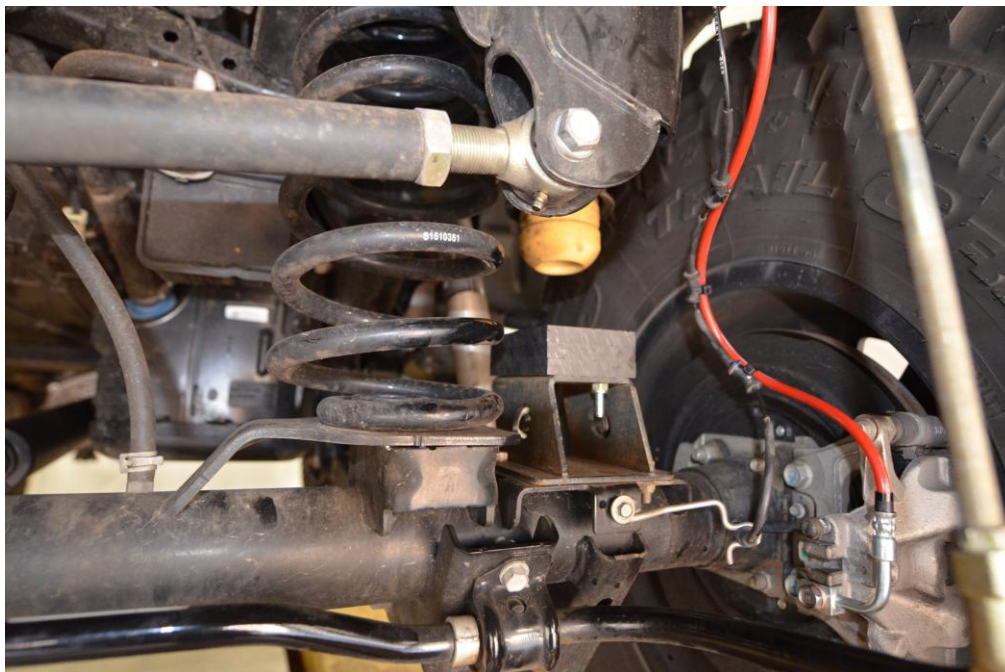
Figure 32: Rear Gladiator Extended Brake Lines installed
