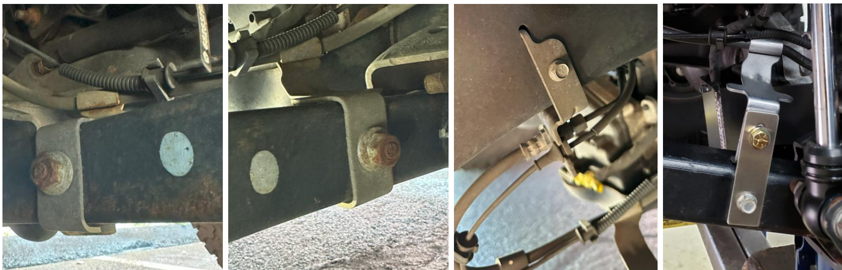
Figure 15: Brake line brackets reinstalled
