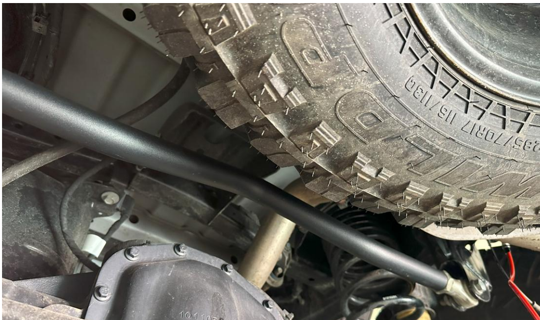
Figure 28: New rear track bar installed
