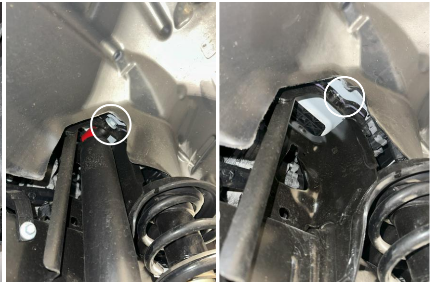
Figure 4: Front upper passenger shock bolt removed
