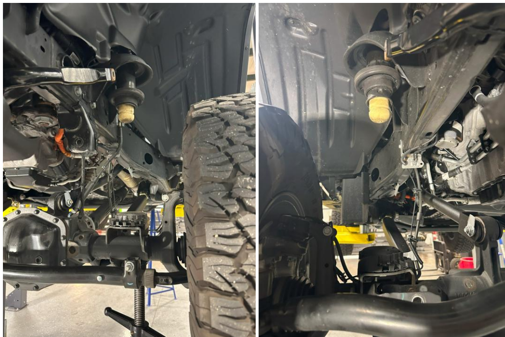
Figure 9: Axle drooped with old springs removed
