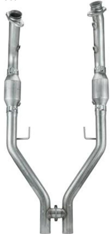
1. Begin by disconnecting your negative cable from your battery, as you will need to unplug and remove your O2 sensor harnesses. Place the vehicle on a lift or four jack stands at maximum height. This will aid in an easier installation. Note: Make sure to support your mid-pipes just past the connection point between the factory h-pipe.
