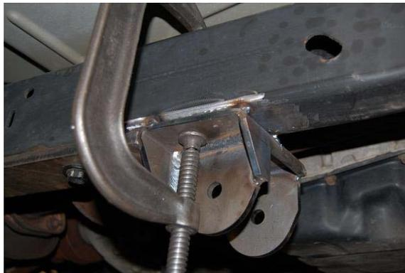
12. Next you will need to prep the driver side frame right above the new lower control arm bracket. You will need to unclip the brakeline, fuel line and any other wires running down the frame in this location. We carefully removed these lines, saving the frame clips as they will be reused. We also wrapped the lines in tin foil to help prevent any weld spatter getting on the lines or wires.
