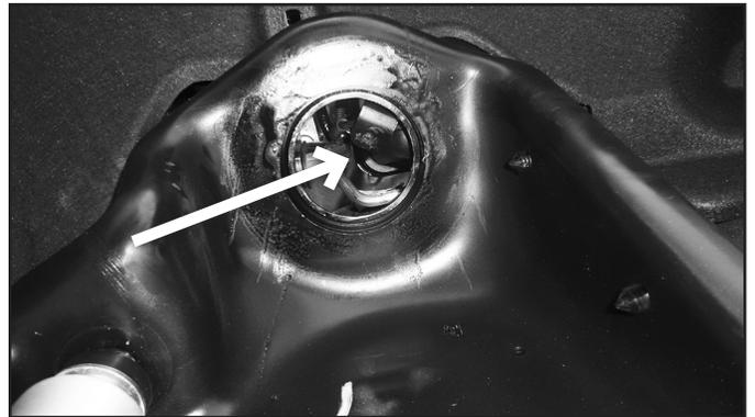
13. Place the upper coilover mounting bracket up to the upper mount. Rotate the bracket so that the reservoir bracket is parallel with the frame. (Fig 6)
