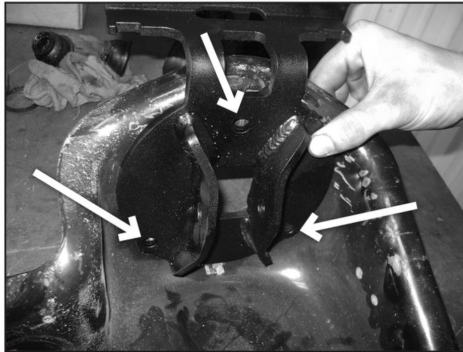
14. Mark the center of the holes, remove bracket, and drill out to 15/32" to 1/2". Make sure the drill does not damage the module on the driver's side (not present on all model year trucks)!
