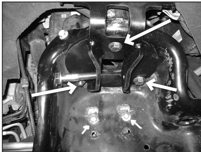
16. Install the lower bracket with new 14mm bolt (#953). Tighten to 75 ft-lbs.
