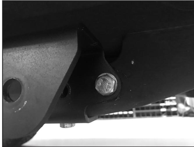
9. The frame bracket should now be installed with hardware left loose (Fig 4).
