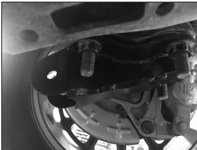
4. Repeat bracket installation on the passenger's side.
