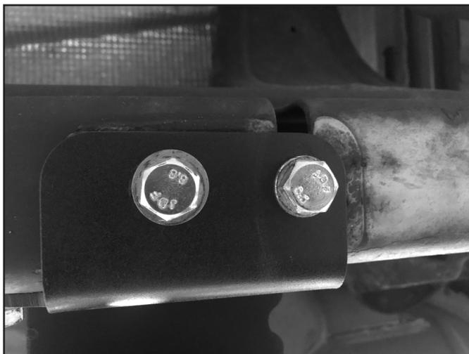
7. Next, insert the nut tab with the 9/16" weld nut into the frame pocket. These are also side specific, make sure the flat face is towards the outside of the vehicle and the slight bend is pointing up.
