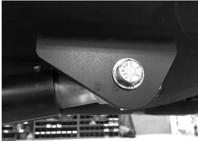
16. At this time, the 9/16" hardware at the frame and axle can be torqued to 90 ft-lbs. All 7/16" hardware can be torqued to 59 ft-lbs.
