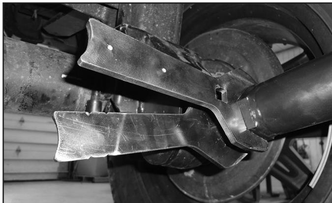
22. Use the levels on the wrench to gauge how much force is inputted into the Recoil Traction Bar. The wrench is designed to be used at the traction bar slider end as shown in Figure 7. Make sure the wrench is pressed firmly against the bushing / tube for an accurate measurement.
