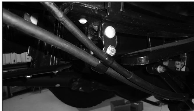
76. Use the two provided wire clips from bolt pack 989 to secure both E-brake cables to the E-brake clamp bracket with the provided 5/16" hardware from bolt pack 989 (Figure 23).
