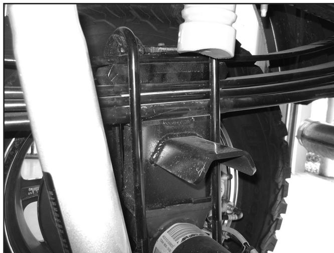
55. Raise the axle to engage the block spring alignment pins. Fasten the entire assembly with the provided u-bolts, washers, and nuts. Snug but do not torque the u-bolts at this time. (Fig 17)
