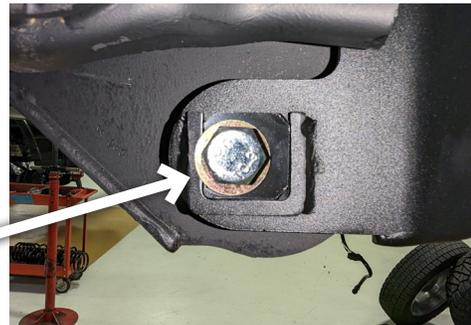
24. Repeat installation of new radius arm on the passenger's side. Tighten axle hardware to 240 ft-lbs (4 plc). Do not tighten the frame mounting brackets at this time. Reattach vacuum lines to new radius arm using provided christmas tree zip ties.
