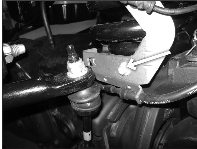
7. Remove the clips holding the front brake lines to the brackets on the frame. Carefully cut the factory bracket so that the brake line can be removed without breaking loose the fittings. Remove the factory brackets from the vehicle. Do not damage the brakeline!
