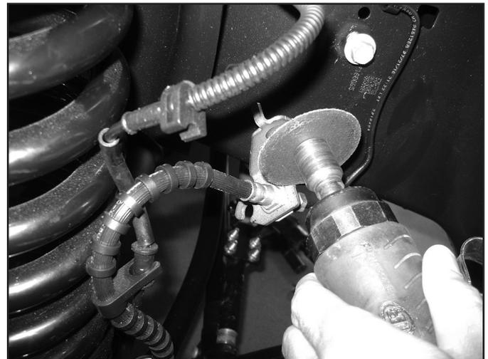
8. Free the hub vacuum lines from the axle to allow for adequate droop (Fig 3, 4).
