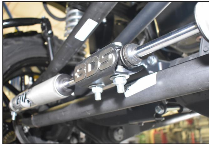
9. The badge can now be riveted on to the front plate using the provided 1/8" rivets. Any residue on the badge can be cleaned up using alcohol or brake cleaner before install. With the badge not installed it can be painted to what ever color you desire, or left raw as a stainless steel badge.
