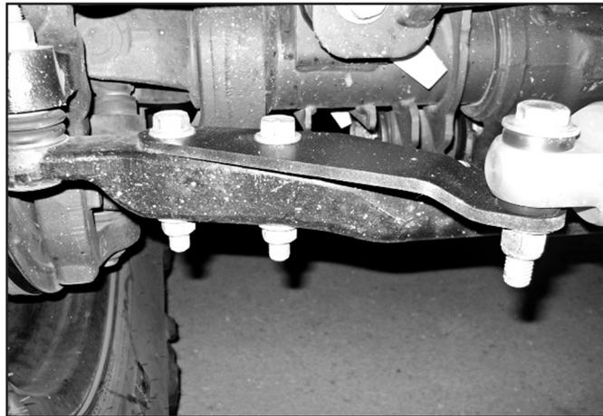
4. Install new center bracket with factory bolts at the bottom side, install new 10mm x 30mm bolts with spacer washers into the top mount. Attach rear axle tube bracket with hardware. Tighten 10mm x 30mm to 30ft-lbs, 12mm x 150mm with 12mm (small OD washers) to 40ft-lbs. (Fig 2a, 2b)
