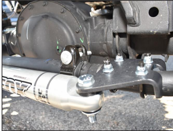
6. Install the driver's side stabilizer bracket to the top side of the tie rod end. Measure the distance between centers of the stabilizer mounts and set the same as the passenger's side. Tighten u-bolt hardware to 20 ft-lbs. Do not over torque, or the bracket may become deformed. (Fig 4)
