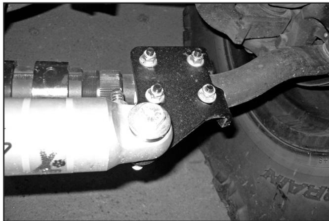
7. Grease and install bushings with sleeves into the steering stabilizers
