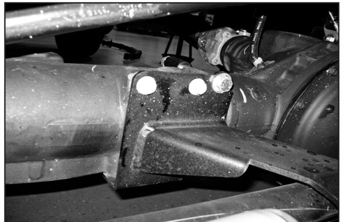
5. Remove the tie rod adjusting bolt and rotate the clamp 180 deg so the bolt is on top. Reinstall the bolt from front to back for stabilizer clearance. (Fig 3)
