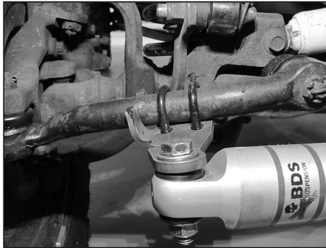
6. Attach driver's side bracket to bottom side of tie rod next to the clamp (Fig 3) with provided U-bolts. Leave hardware loose.
