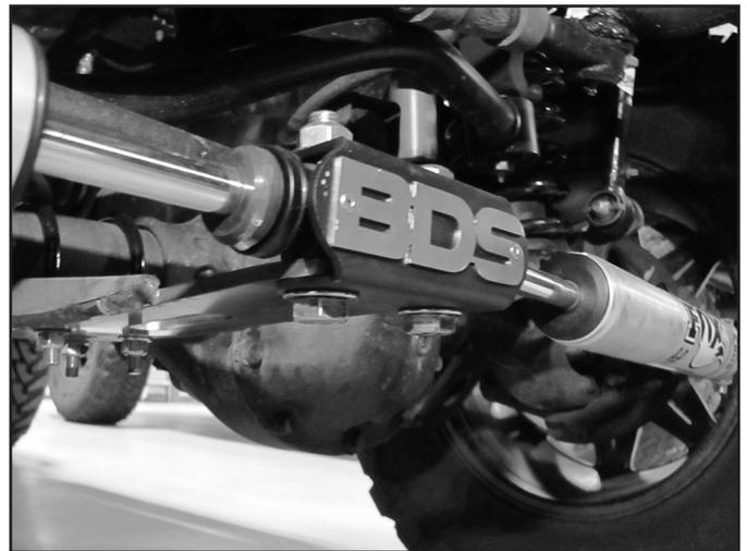
8. The badge can now be riveted on to the front plate using the provided 1/8" rivets. Any residue on the badge can be cleaned up using alcohol or brake cleaner before install. With the badge not installed it can be painted to what ever color you desire, or left raw as a stainless steel badge.
