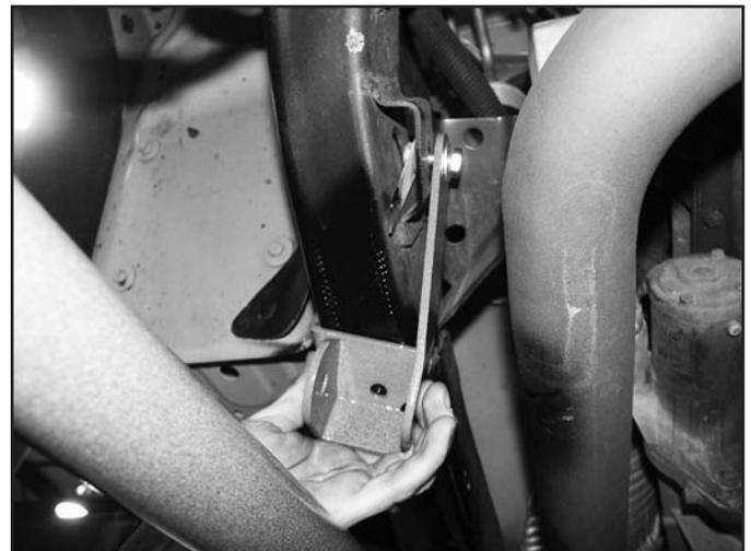
23. Drill 3/8" holes at the two marks on the outside surface of the frame. Drill the holes all the way through the frame.
