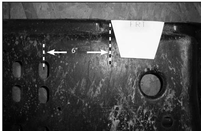
7. **03-06 Models:** This trimming procedure is to be done on the rear driver's and passenger's side corners of the skid plate.
