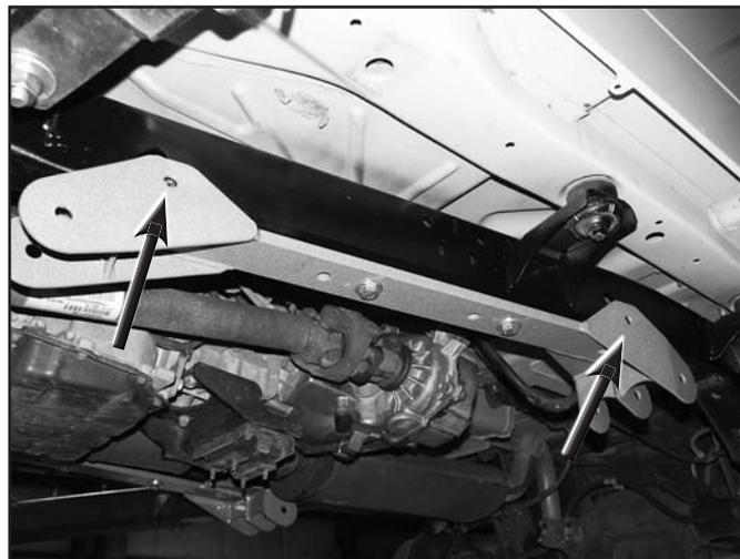
10. Remove the subframes and drill 7/16" holes at the marks on the frame. Take care to drill the holes straight (square) to the frame. Drill through both the outer and inner surfaces of the frame. Caution: Check for lines and hoses on the inner frame rail before drilling.
