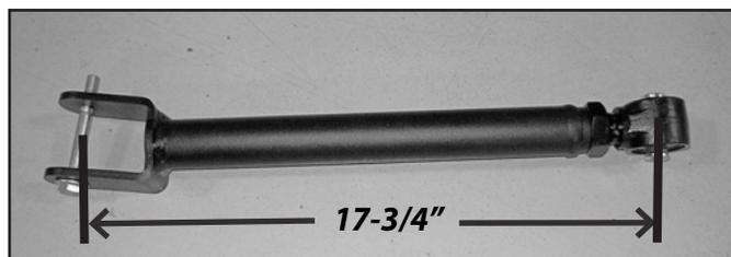
29. Install the new upper control arms in the new upper control arm brackets with 7/16" x 3" bolt, nut and 7/16" SAE washers (BP 731). Attach the arm to the OE front axle mount with the 10mm x 90mm bolt used earlier along with a 10mm nut and 3/8" USS washers (BP 731). Leave control arm hardware loose.
