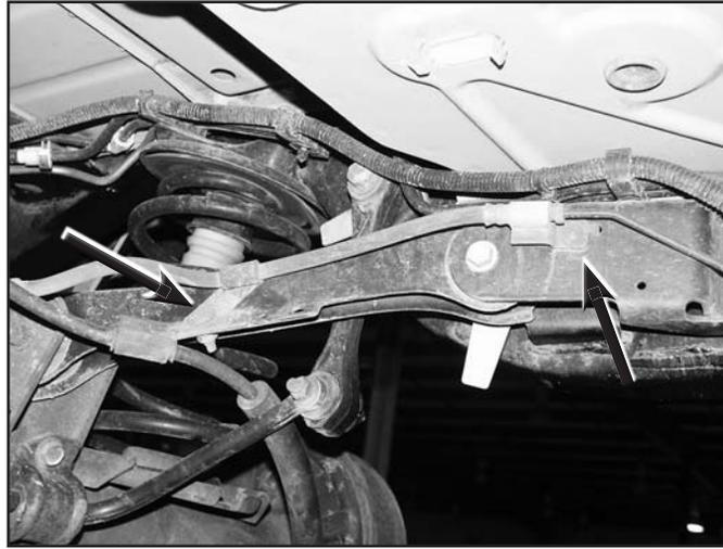
7. Locate (2) remaining lower control arms (A220). Adjust the length to 29-1/4". Install a provided 90° grease zerk (60107) in the flex end so it faces 45° from facing down the arm and towards the outside of the vehicle. The arms are installed with the flex eye at the frame with the bend towards the inside of the vehicle.
