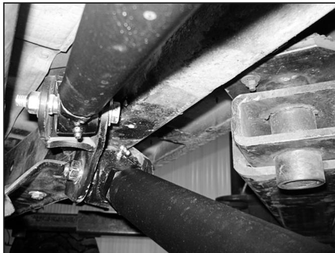
12. Locate the OE mounting tabs on the two emergency cables (Fig 13). Using a cut-off wheel, etch the side of the bracket so that it can be easily formed open and removed from the cable. Leaving the cable free at these points will eliminate the chance of binding during extreme suspension articulation. Take care not to cut into the cable.
