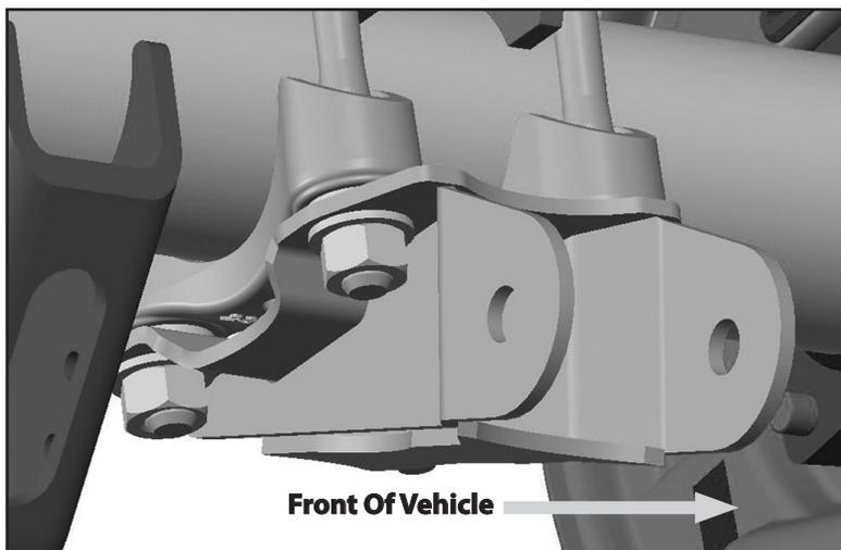
6. Repeat bracket installation on the passenger's side.
