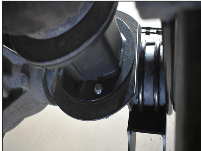
4. Install the U-Bolts through the slots in the axle mount bracket (03854), attaching the 1/2"-fine thread nuts and 1/2" SAE Washers to the U-Bolts from Bolt Pack 962. The axle mount bracket should cradle the axle. Make sure the mounting tabs on the bracket are facing towards the front of the vehicle. Do not tighten hardware at this time.
