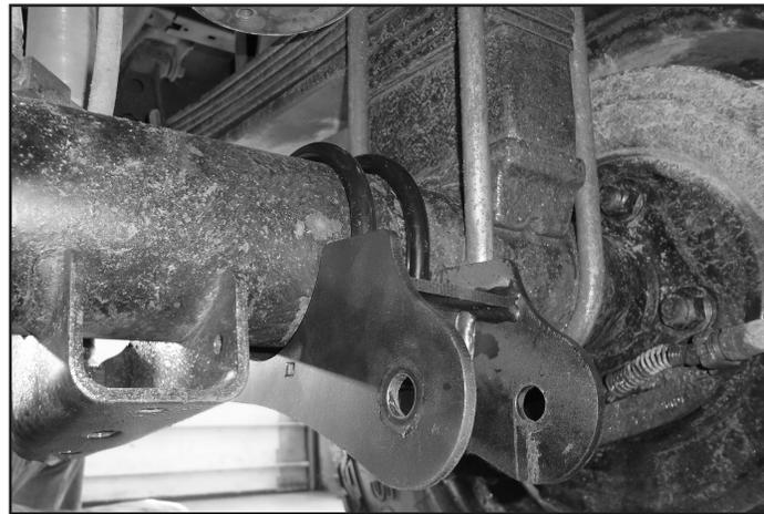
8. Repeat axle bracket installation on the passenger's side of the vehicle.
