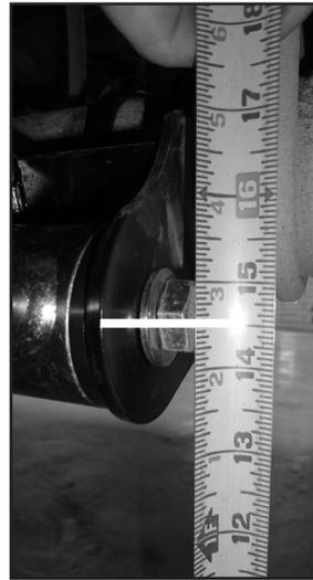
7. After the axle bracket is set at the correct height, tighten the 1/2" nuts on the axle bracket to 45 ft-lbs
