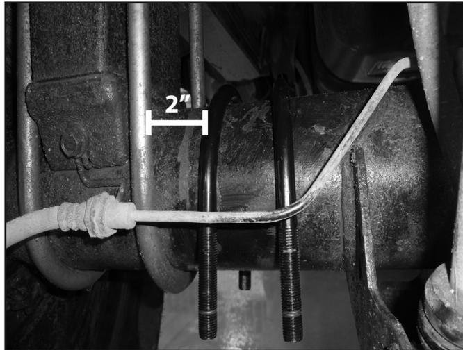
3. **Rear Air Ride Only:** It may be necessary to grind the factory air bag mount a little to allow the U-bolts to sit square. The axle bracket will sit flush against the block U-bolt.
