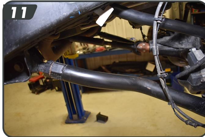
**HINT:** If mounting bolt is difficult to install due to misalignment of the control arm bushing with mounting bracket, either <sup>(1)</sup> adjust height of axle housing with hydraulic jack, or <sup>(2)</sup> move axle housing into position with a heavy-duty ratchet strap.
