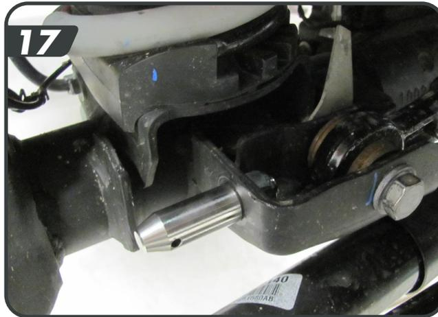
ao. Install the longer disconnect post on the driver side axle sway bar link mount with it pointing inboard [18]. Fasten with the  $\frac{1}{2}$ " nylock nut and tighten to 64 ft-lbs. Tighten the post with the pin hole parallel to the ground. Slide the polyurethane spacer on the pin up against the axle tab.
