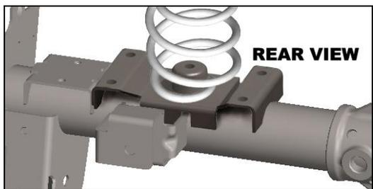
**IMPORTANT:** Adjustable Spring Mount bracket must be installed with rounded side facing forward and flat side facing the rear as illustrated above.
