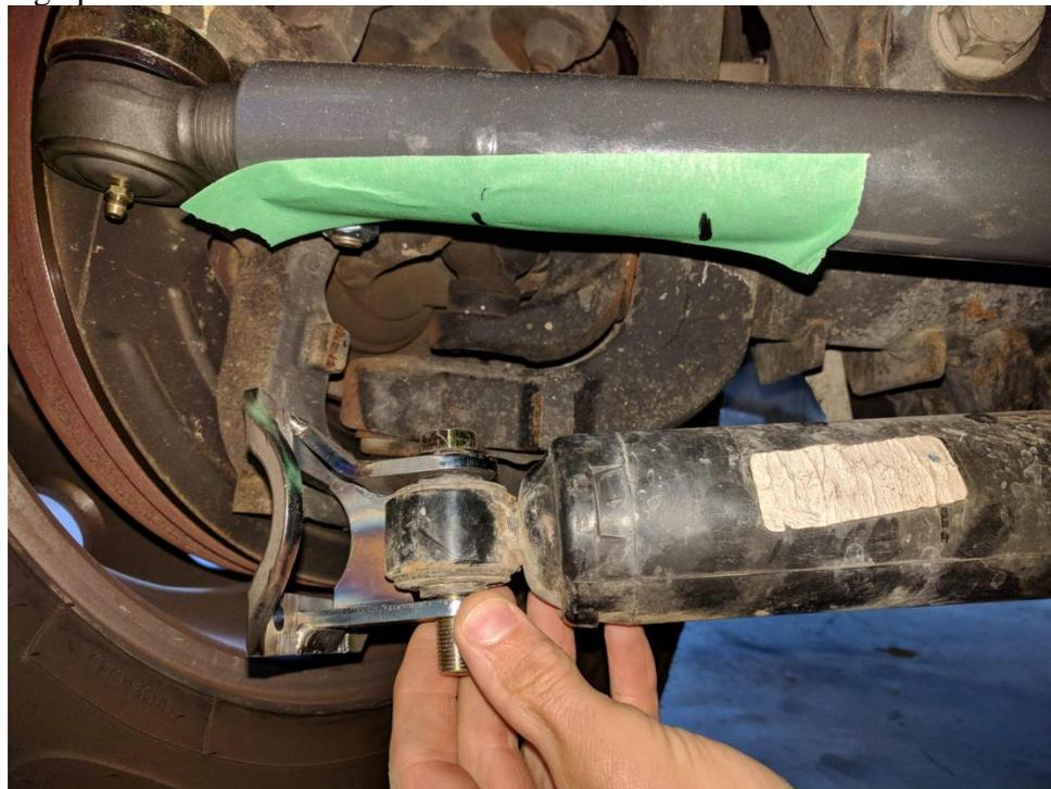
**Figure 3. Correct Orientation of Steering Stabilizer Clamp**
