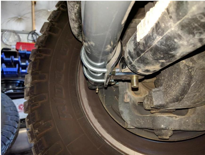
**Figure 5. Clamp Installed with Bolt Perpendicular to Ground**
