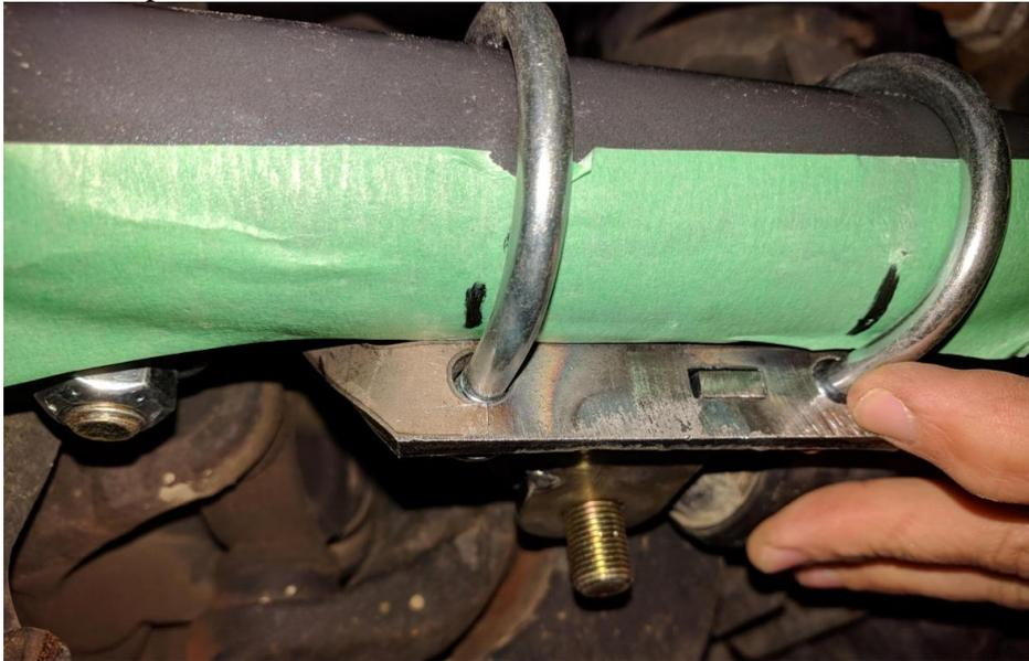
**Figure 4. Clamp Centered on Tie Rod**
