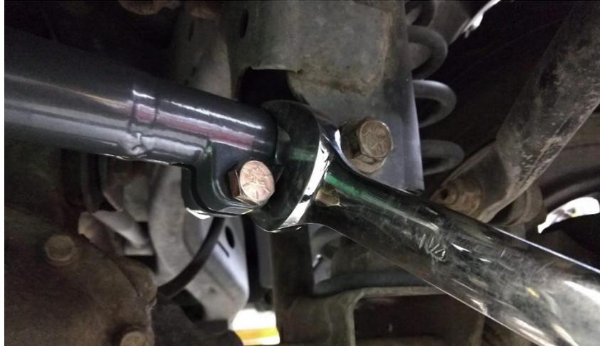
**Figure 7. Adjusting the Track Bar to Center the Axle**
