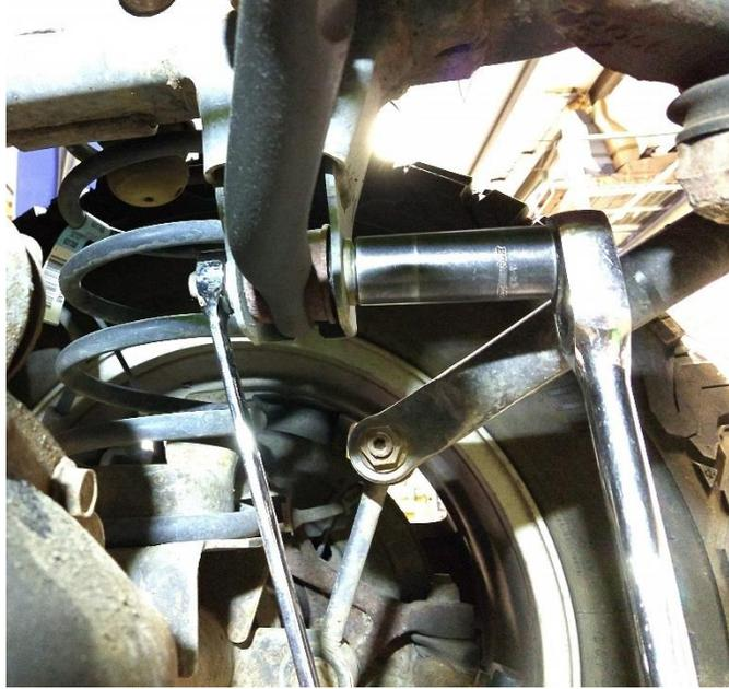
**Figure 3. Removing the Track Bar from the Frame Side**
