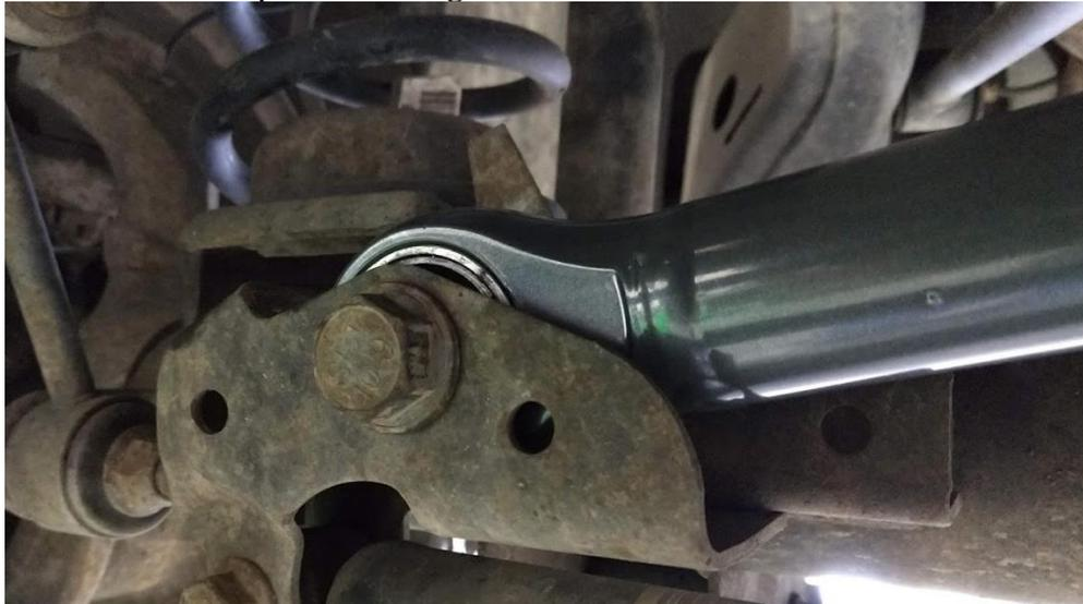
**Figure 4. Synergy Mfg Track Bar Installed at the Axle**
