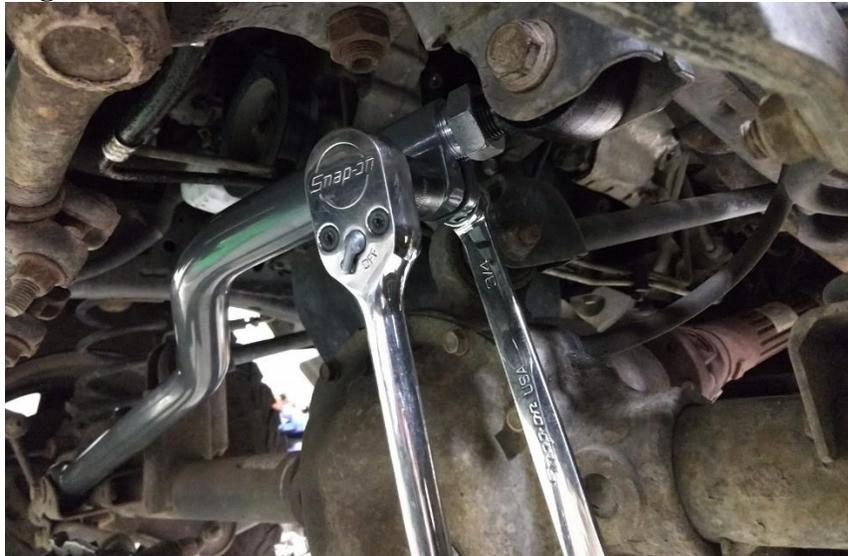
**Figure 8. Tightening the pinch bolt and nut.**
