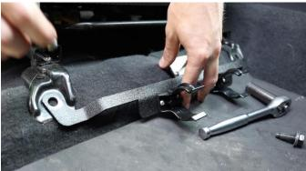
The seat safety rated torque specifications for each bolt is 27ft-lbs.
