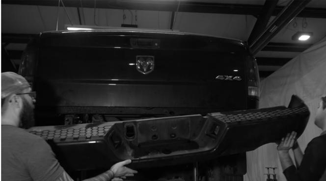
Remove the sensors and sensor wiring harness. Remove the trailer plug. Remove the license plate lights.
