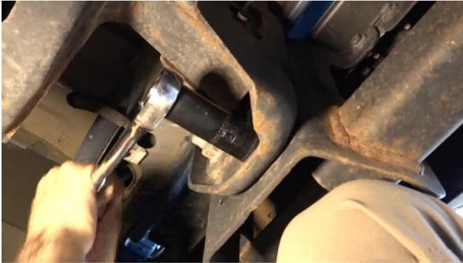
Disconnect your hitch plug and license plate lights, and with a clip remover tool, free the power harness from the bumper.
