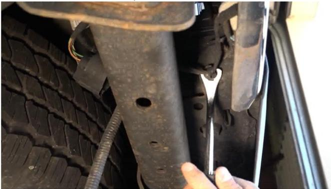
Remove the bumper. With a 13mm socket, remove your hitch retaining plates and hitch.
