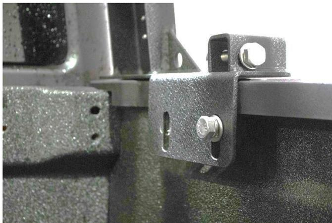
Use the included Hex bolts, lock washers, flat washers, and thread locker and secure the Bed Rack down into the T-Nuts.
