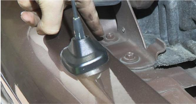
Place the side specific bracket onto the top of the hinge, and secure it by reusing the factory hardware.
