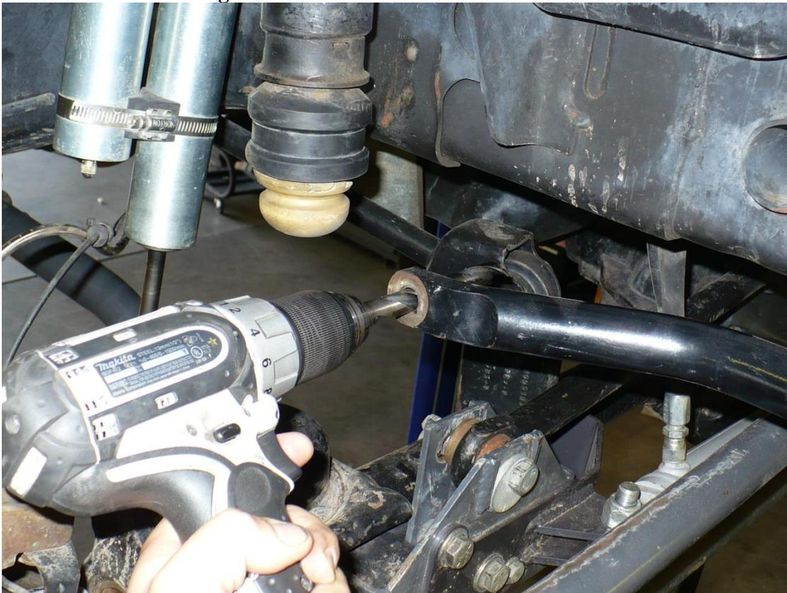
**Figure 1. Drilling Out the Sway Bar**
